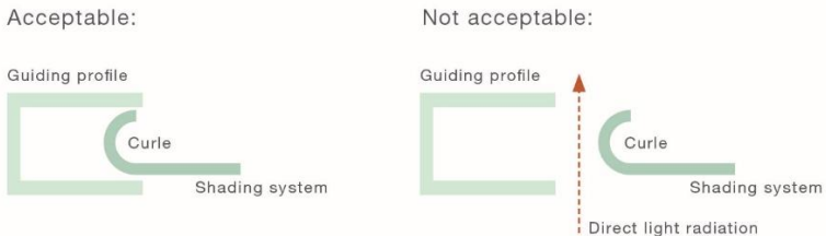
Figure 16: Evaluation of rolling in of free hanging edges
